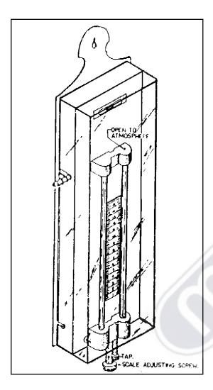
Water Gauge comprises two nos. 6mm straight corning glass tubes terminating into a brass block with a connecting passage. One limb is open to atmosphere & other is connected to fan drift. A tap is provided to close the connection while taking reading. A scale with adjusting screw is mounted behind the glass tubes. A sprit level helps in keeping the instrument vertical.
